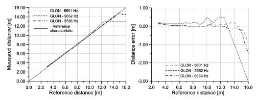
Fig. 5. Characteristics of errors of distance measurement with a GLOP2 locator - laboratory tests.
