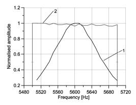
Fig. 2. Frequency characteristics of the course of analogue and digital signal processing within the frequency band 5500 Hz - 5700 Hz. 1 – actual characteristics, 2 – corrected characteristics.
