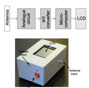
Fig. 1. Block diagram and photograph of GLOP2 locator.
