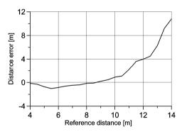
Fig. 7. Errors of distance measurement for three GLON transmitters obtained in measurements in the vicinity of large metal objects.
