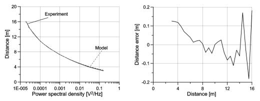
Fig. 3. Static characteristics of the locator: experimental, model and error of characteristics modelling.
