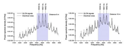
Fig. 4. The result of estimation of spectral density of the signal coming from three GLON transmitters with frequencies of 5536 Hz, 5601Hz and 5652 Hz, received from a distance of 8 m and 16 m.
