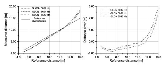
Fig. 6. Characteristics of errors of distance measurement with GLOP2 locator – tests at the coal mine BOBREK, depth 723 m.
